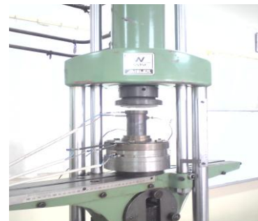
Figure (2): Photograph of heated circular die and punch apparatus.
