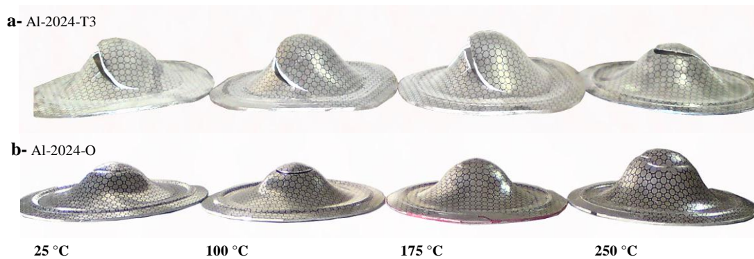
Figure (5): Punch stretch experimental results at several temperatures for Al-2024-T3 and Al-2024-O
