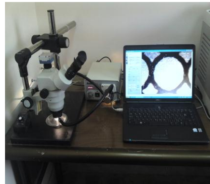
Figure (3): The equipment of the optical strain measurement system.
